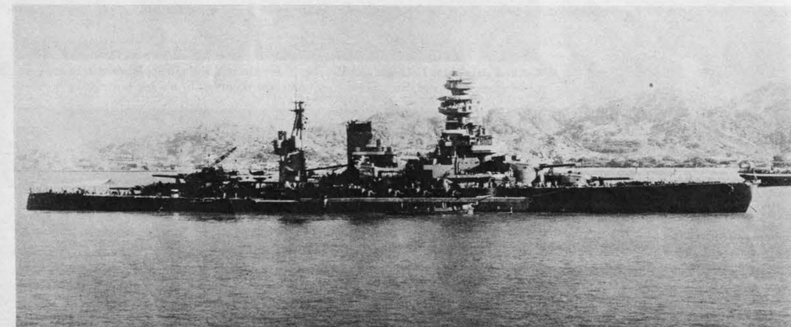
Nagato Class was Japan's best at the outbreak of hostilities. Heavy tripod foremast on which her pagoda is built is visible between the numerous control platforms. The use of tall superstructures by the Japs provides excellent visibility but limits the arc of antiaircraft fire.
